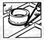
Use a good sharp model knife to trim and detach plastic parts. Some parts will appear to have extra "tabs" on them — cut these off.
