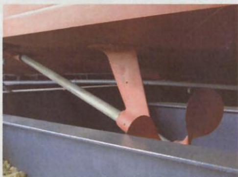
Above: the stern of Lt. Kennedy's PT 109. Left: butterfly valves routed the exhaust either directly out or through the muffers. Below: port screw shaft.
