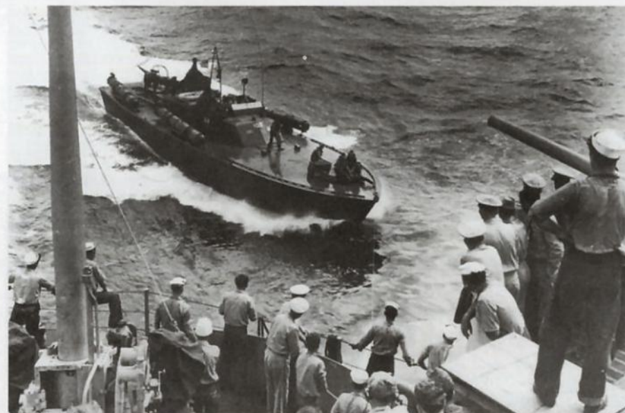
Previous page: PT 103, the first ELCO 80 footer, pictured during sea trials. Over 300 boats of similar design were built during World War II.
