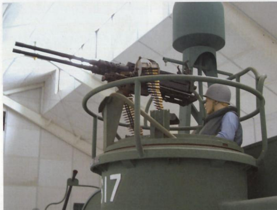
Above, and below: the forward hydraulic turret was offset to starboard. Right: note the late type radar mast.
