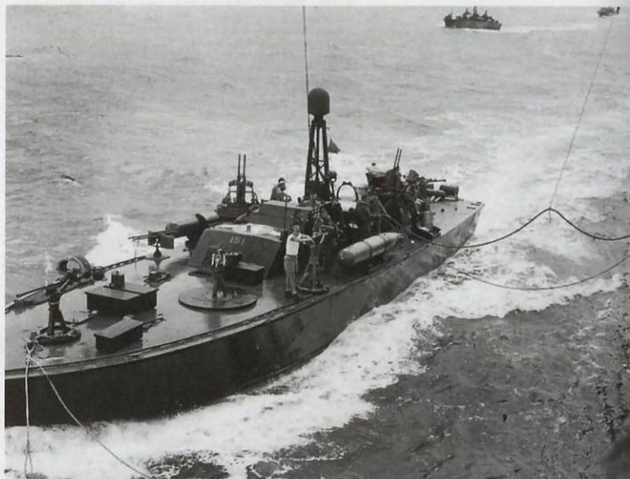
Above: PT 191 refuelling at sea from a tender. Such operations were usually accomplished while underway.
