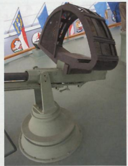
This page: the fore 37mm gun on a Mk.1 mount. This is just an approximate replica, nevertheless gives a general idea of the layout of this weapon.
