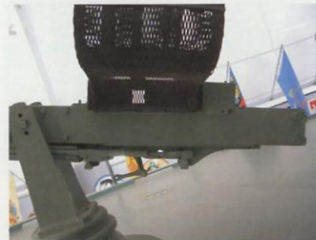
This page: the fore 37mm gun on a Mk.1 mount. This is just an approximate replica, nevertheless gives a general idea of the layout of this weapon.
