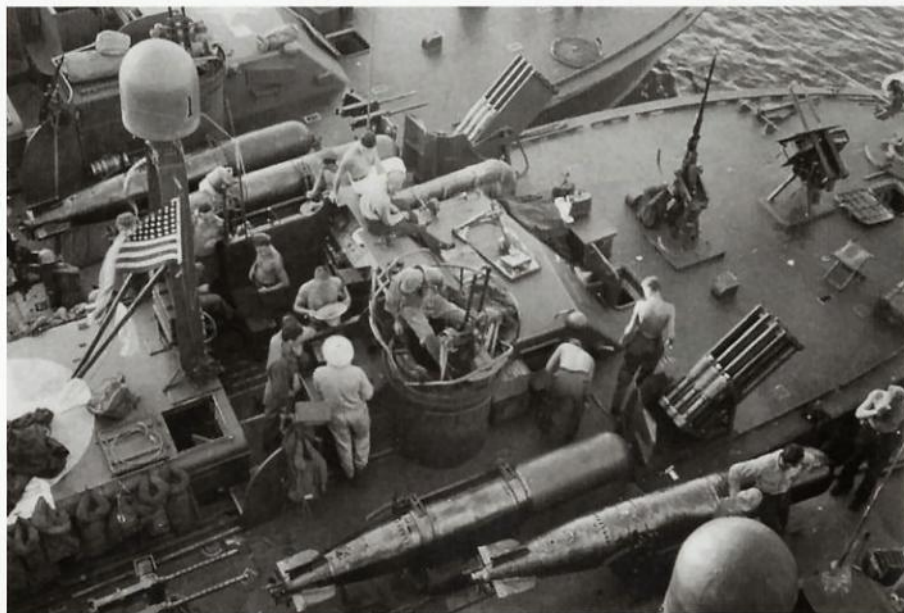
Above: note the early rocket rails on PT 131, and the life vests hanging on the deck house.
