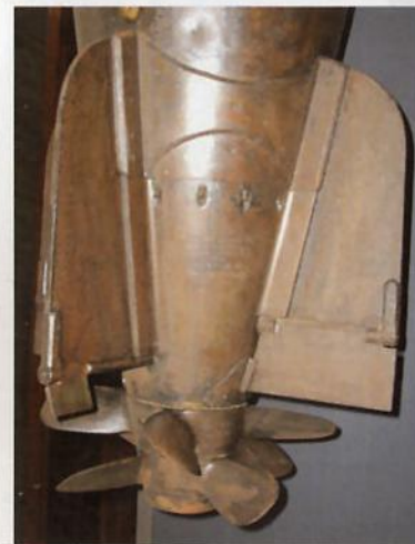
Above: early tube-type torpedo launcher. Left: Mk.XIII torpedo fins and screws. Below: smoke generator on the stern.
