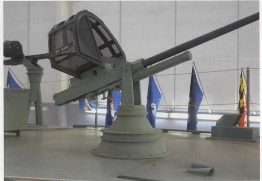
This page: the fore 37mm gun on a Mk.1 mount. This is just an approximate replica, nevertheless gives a general idea of the layout of this weapon.
