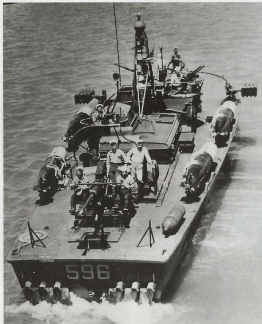
Previous page, and above: bow and stern views of PT 596 with the rocket launchers deployed and all deck details clearly visible. She represents the final configuration of WWII ELCO PT boats.
