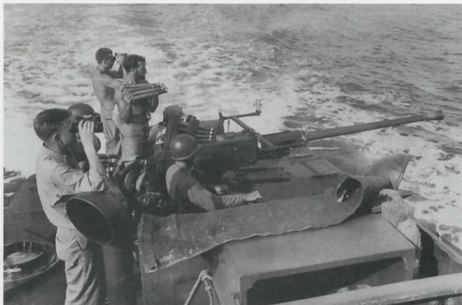
Pages 38 and 39: the heaviest artillery carried by the PT boats was the 40mm Bofors gun. It required a crew of four.
