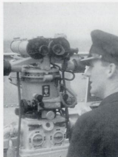
The binocular 7x50 used on the RZ5 torpedo targeting director mounted on the top of the armoured bridge.
