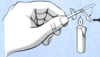
flame and pull it both ways. Stretch the antenna as follows with reference to the drawings, etc. Cut the string a little longer than necessary. Fix it in place by applying adhesive with a match. The extra length should be cut off after the adhesive has dried.
